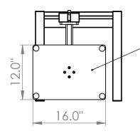
Plaform can be rotated 90° so that width and depth are interchangable
