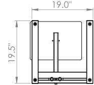
The Sound Anchor ADJ4 upright can be moved and locked down anywhere along a slot that runs the width of the stand.
